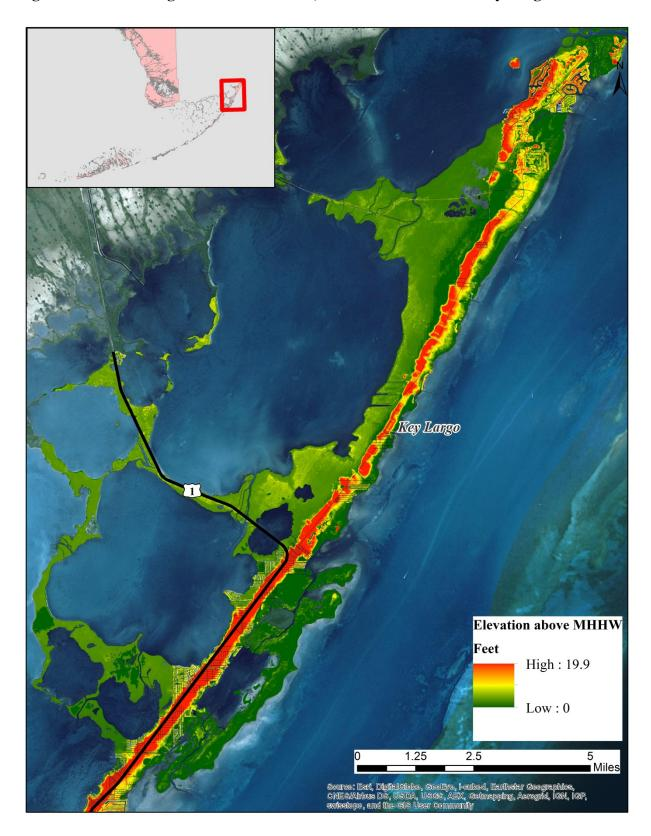
Figure 2a. MHHW Digital Elevation Model, Northern and Central Key Largo
