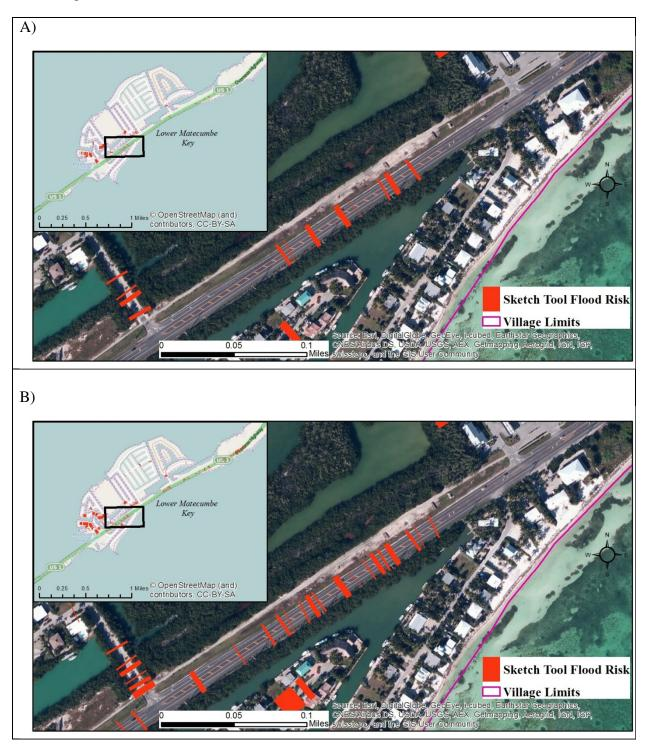
**Figure 16b:** FDOT Sea Level Rise Sketch Planning Tool Close-Up for US1, Lower Matecumbe Key, 2060 Sea Level Rise Scenarios. Picture A) shows road segments predicted as vulnerable to nuisance flooding with 9 inches of sea level rise (2060, Low Scenario). Picture B) shows road segments predicted as vulnerable to nuisance flooding with 24 inches of sea level rise (2060, High Scenario).
