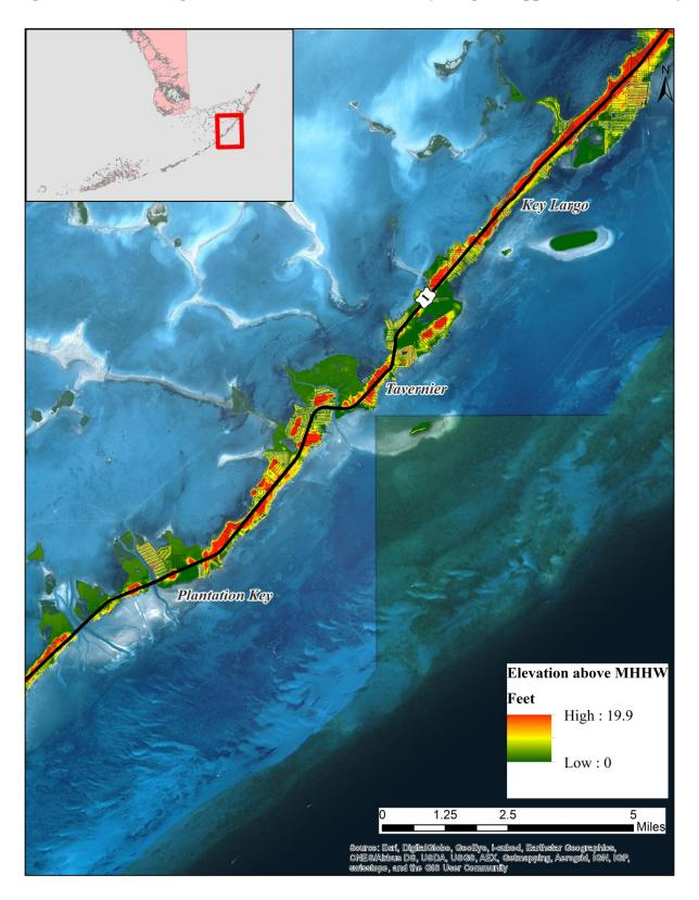
Figure 2b. MHHW Digital Elevation Model, Central Key Largo to Upper Matecumbe Key
