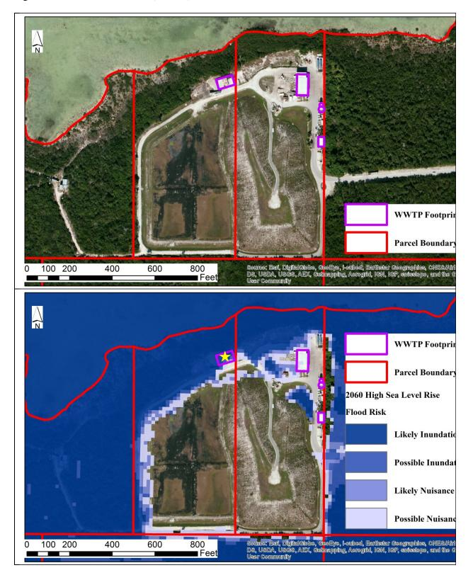
**Figure 12**: Layton Wastewater Treatment Plant. Aerial photograph (top) and 2060 high sea level rise assessment (bottom). Yellow star indicates structure with flood risk.
