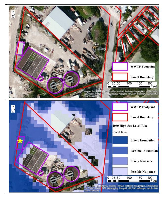
**Figure 8**: Key Haven Wastewater Treatment Plant. Aerial photograph (top) and 2060 high sea level rise assessment (bottom). Yellow star indicates structure with flood risk.
