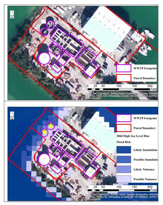
**Figure 11**: **Cudjoe Regional Wastewater Treatment Plant.** Aerial photograph (top) and 2060 high sea level rise assessment (bottom). Yellow star indicates structure with flood risk.
