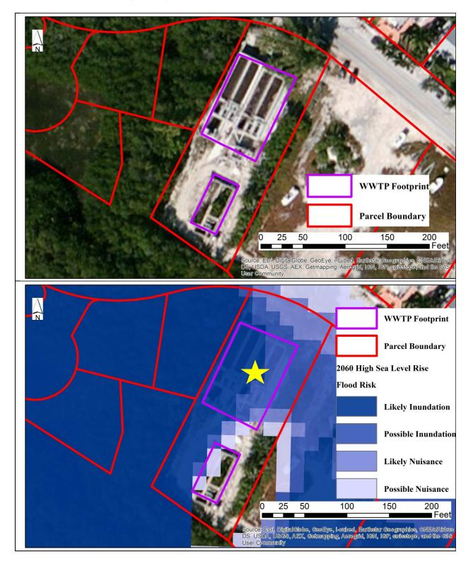
**Figure 9**: **Bay Point Wastewater Treatment Plant.** Aerial photograph (top) and 2060 high sea level rise assessment (bottom). Yellow star indicates structure with flood risk.
